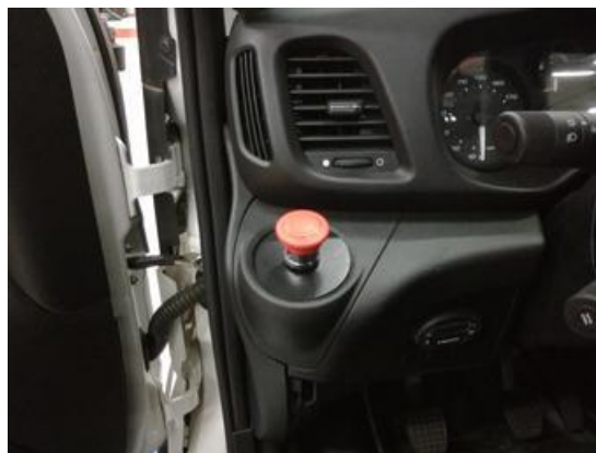
Figure 2-4 HV Emergency Shut down Installation
