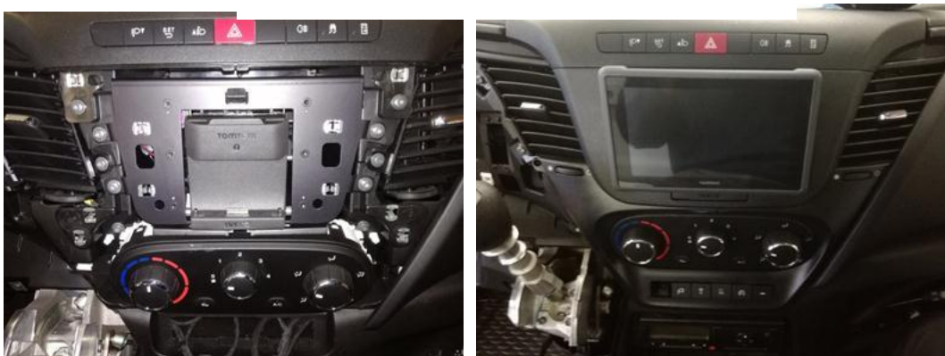
Figure 2-11 HMI Installation Step 3 (Cradle) – Step 4 (TOM-TOM)
